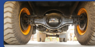
▲ Rugged front axle for guaranteed best traction during crane operation.
