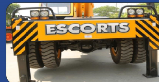
▲ Front outrigger with rectangular outer box for better load lifting, stability & safety. Front working light for better vision.
